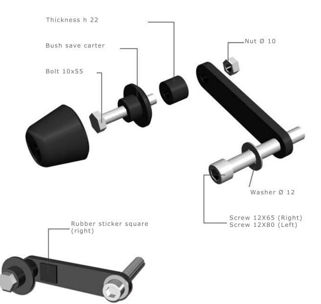
SEARCH AND FIND THE FIXING POINTS ON THE MOTORBIKE BEFORE START TO MOUNTAIN, USE THE SPECIFIC THICKNESS AND BOLTS LIKE DESCRIBED IN THE PICTURE (SO YOU CAN GET THE RIGHT PROMINENCE FROM THE MOTORBIKE). FIX THE PVC HEAD AFTER FIXED AND TIGHTEN ALL THE KIT ONLY.
